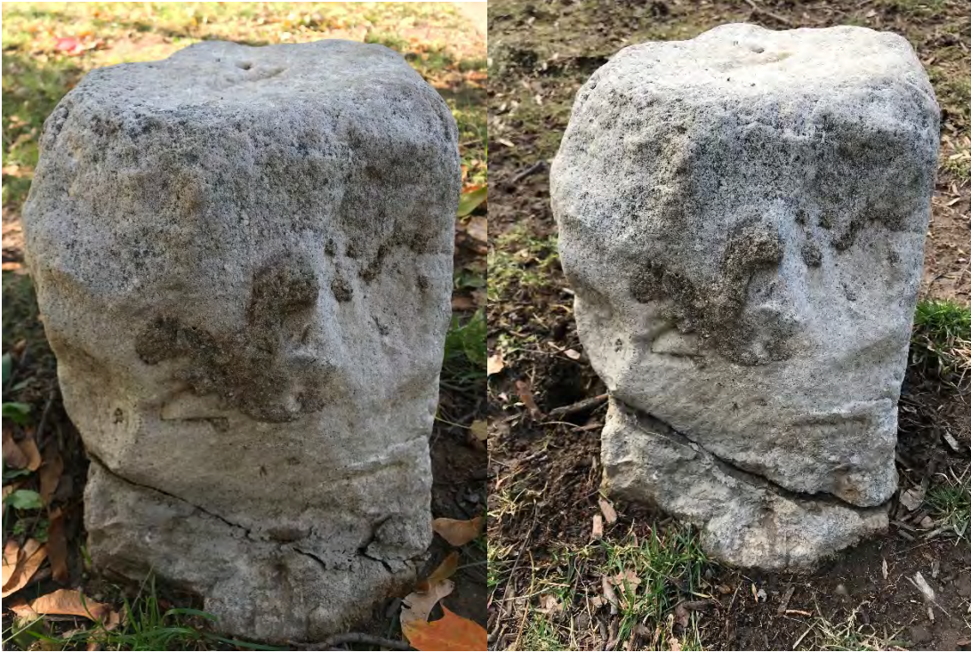
Figure 37: The back of OBS 23 on Dec. 31, 2019 (left) and March 25, 2020 (right) showing shifting of the stone. It was probably hit by a riding lawn mower or snowplow.
