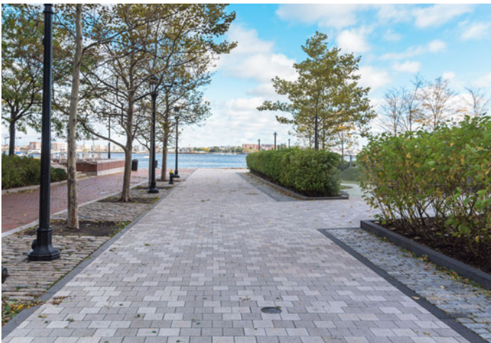
Use of light coloured pavers to reduce urban heat island effects while maintaining contrast between walkway and furnishing zones
