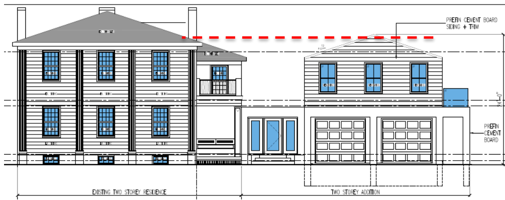
FRONT ELEVATION – the 2-storey garage will be separated from the heritage building by a 1-storey link with a flat roof and a concrete slab foundation to avoid impacts to the roof or foundation of the heritage building. [2M Architects]
