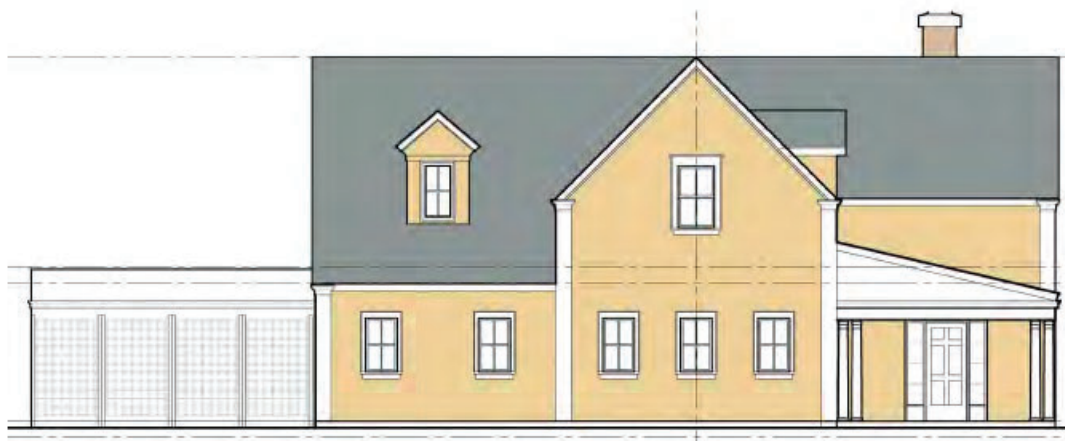
50. Drawing of the typical left elevation of the proposed Front Gable Residences. (Giannone Petricone Associates and ERA, 2021).
