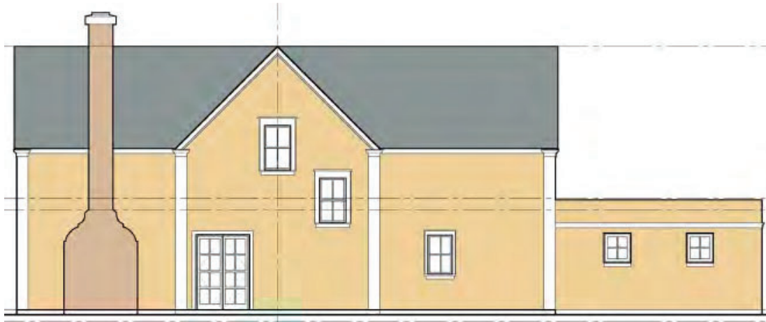
49. Drawing of the typical right elevation of the proposed Front Gable Residences. (Giannone Petricone Associates and ERA, 2021).
